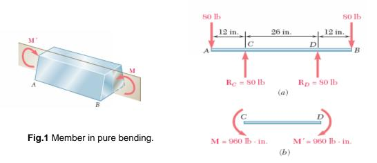
Fig. 2 Beam in which portion *CD* is in pure bending.
