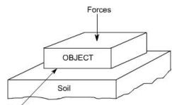
Another type of simple stress is the **bearing stress**, it is the contact pressure between two bodies. (It is in fact a compressive stress).
