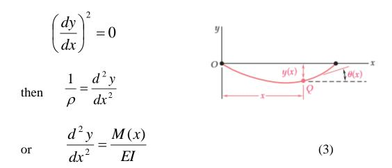
Multiply both sides by EI which is constant and integrating with respect to x:
