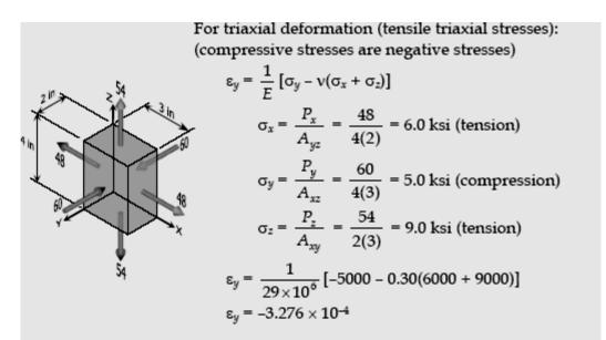
$\varepsilon_y$  is negative, thus tensile force is required in the *x*-direction to produce the same deformation in the *y*-direction as the original forces.
