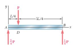
Fig. 9.27 Free-body diagram for beam of Fig. 9.16.
