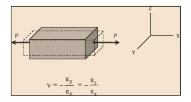
where  $\varepsilon_x$  is strain in the x-direction and  $\varepsilon_y$  and  $\varepsilon_z$  are the strains in the perpendicular direction. The negative sign indicates a decrease in the transverse dimension when  $\varepsilon_x$  is positive.
