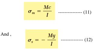
Equations (11) and (12) are called the *elastic flexure formulas*, and the normal stress  $\sigma_x$  caused by the bending or "flexing" of the member is often referred to as the *flexural stress*. We verify that the stress is compressive ( $\sigma_x > 0$ ) above the neutral axis (y > 0) when the bending moment M is positive, and tensile ( $\sigma_x < 0$ ) when M is negative.
