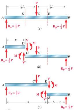
Cutting, now, the beam at a point E between C and B and considering the free body EB (Fig. c), we write that the sum of the vertical components and the sum of the moments about E of the forces acting on the free body are zero. We obtain:
