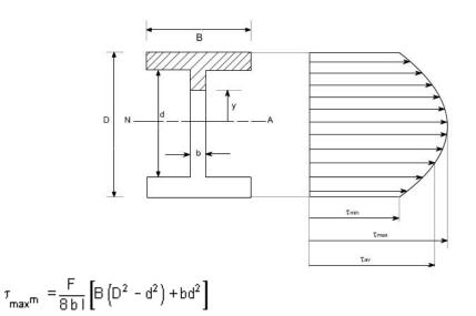
Note: from the above distribution we can see that the shear stress at the flanges is not zero, but it has some value, this can be analyzed from equation (1). At the flange tip or flange or web interface y = d/2. Obviously then this will have some constant value and then onwards this will have parabolic distribution.
