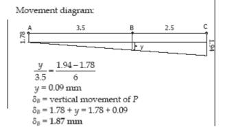
Example 207: The rigid bars AB and CD shown in Fig. P-214 are supported by pins at A and C and the two rods. Determine the maximum force P that can be applied as shown if its vertical movement is limited to 5 mm. Neglect the weights of all members.
