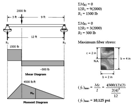
Stress in a fiber located 0.5 in from the top of the beam at midspan:
