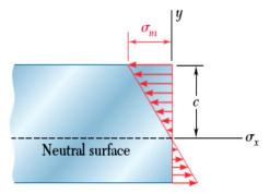
Fig. 5 Bending stresses.
